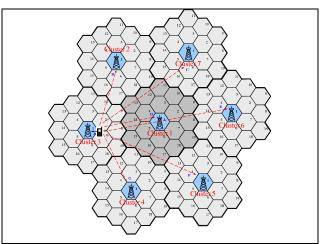
Figure 17.MS uses the same frequency to communicate with all cluster's BSs
