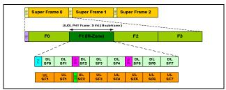
Figure 1 (b) Control channel structure for FDD
